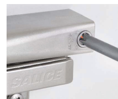
Rotate the screw toward the plus sign to decrease closing speed, or to the minus sign to increase closing speed
